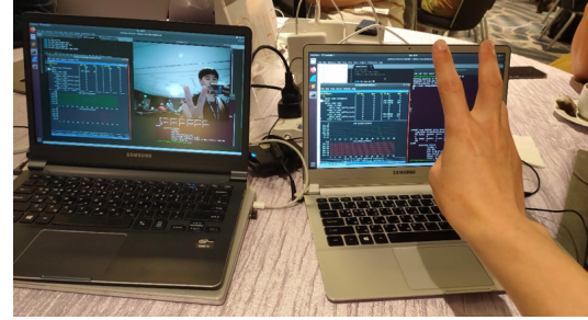
Fig. 5. Webcam streaming experiment by two OCB-mode enabled laptops.
